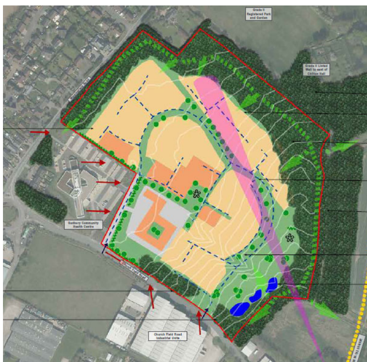
Figure 4: JBA Landscape Strategy extract, to illustrate proposed planting and infrastructure links within the plantation, 20m-26m from the boundary of Chilton Hall. 18.5m depth of trees to the northern boundary are to be removed from G3 to facilitate development.
