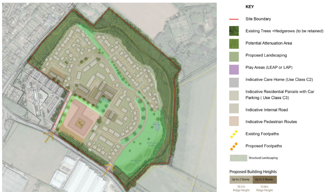
Figure 3: KLH Parameters Drawing overlaid with the Indicative Masterplan to show the height an extent of development, encroaching 18.5m into the G3/G7 plantation along the northern boundary with Chilton Hall.
